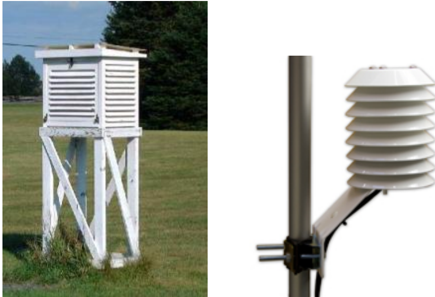
Figure 2: Examples of a Stevenson Screen and gill-type radiation shield for air temperature monitoring
