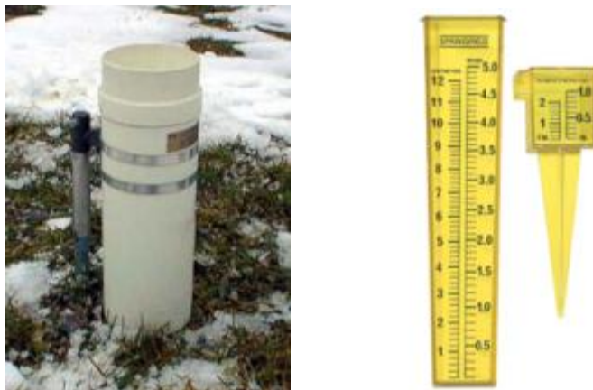
Figure 4: Standard (very accurate) Environment Canada Type B manual rain collector and small diameter (less accurate) rain gauges
