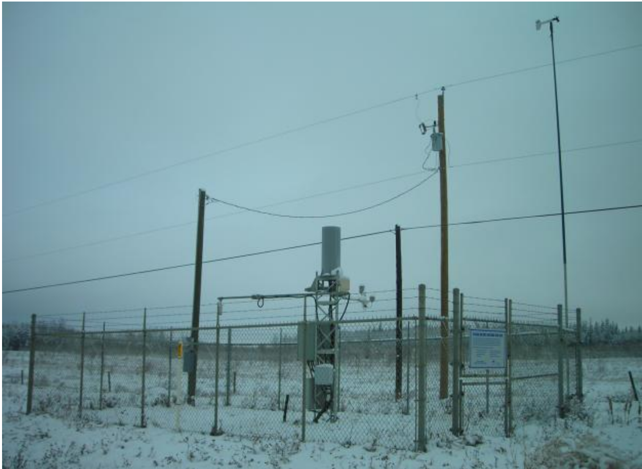
Figure 10: Example of a road weather station (Braden Road). Photo courtesy of Simon Walker.
