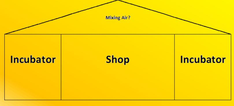
The air in these incubators was mixing with the air in the shop and unintentionally exposing workers.
